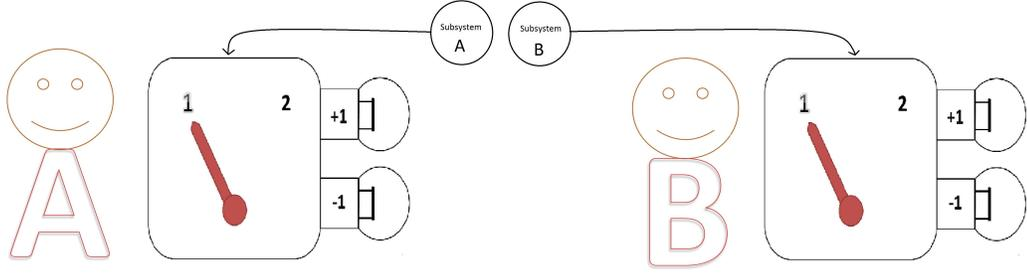
Figure 2.1: Alice on the left and Bob on the right receive subsystem A and B respectively. Each of them is able to choose freely one of the two independent measurement settings as indicated by the red arrow. There are two possible measurement outcomes as indicated by the bulbs.
